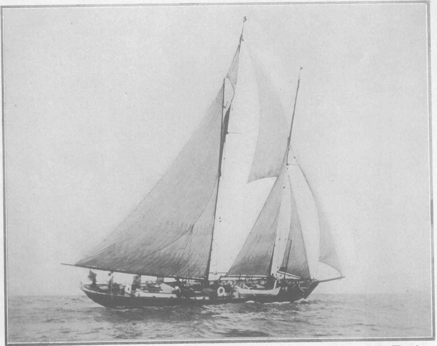
Halcyon is 88 feet over all and was designed by Ford, Payne & Sweisguth. She is owned by Robert and Erwin of Milwaukee, Wisconsin. She has a 100 hp. Kahlenberg oil engine
